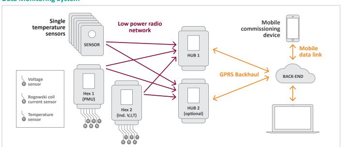
The Hub (KHB) acts as low power radio concentrator, with cellular modem. There may be several Hubs in a remote site to cover large substations and severe shadowing situations. KHB01 is a battery powered monitoring unit for data logging. KHB02 provides for real time alarms and data logging. It requires external powering.
