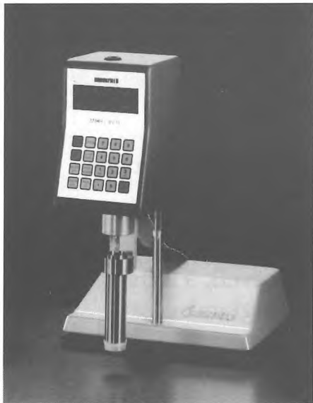
DV-III PROGRAMMABLE FOR SAMPLE TESTING & DATA ANALYSIS
