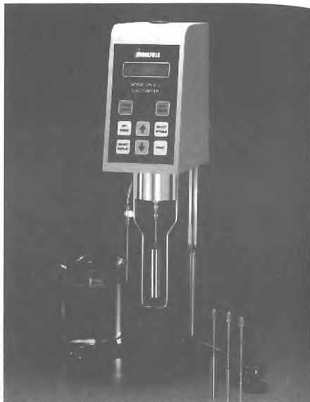
DV-II+ FOR SIMULTANEOUS MEASUREMENT OF VISCOSITY & TEMPERATURE
