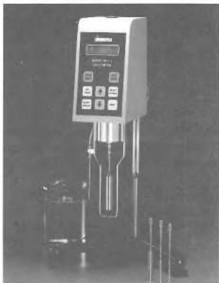
DV-II+ FOR SIMULTANEOUS MEASUREMENT OF VISCOSITY & TEMPERATURE
