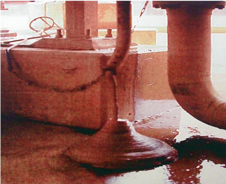
Figure 5: Mineral waste produced with a compression thickener
