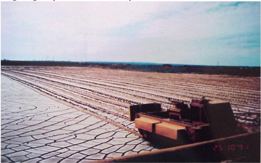
Figure 4: Alcoa Western Australia, bauxite waste dry stacking
