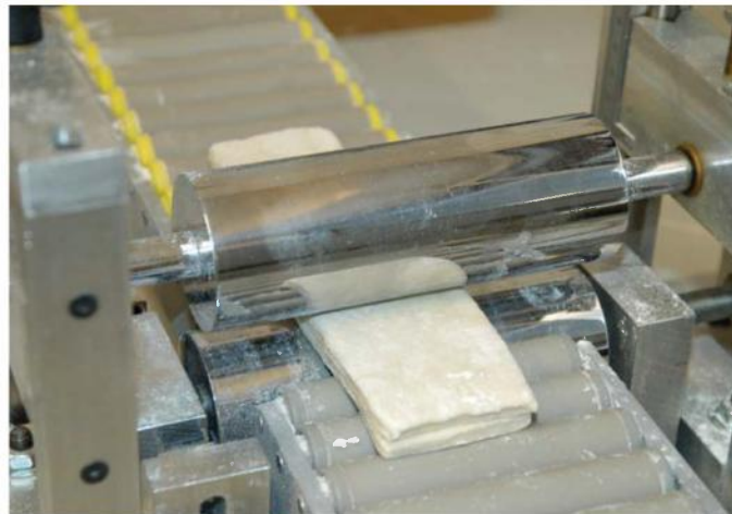
Figure 6: Small scale rig to study the rolling process of dough.
