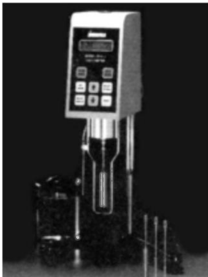
DV-II+ FOR SIMULTANEOUS MEASUREMENT OF VISCOSITY & TEMPERATURE
