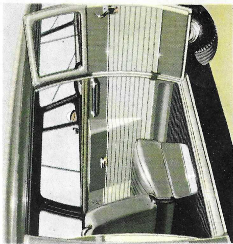
The top-hinged door in the rear enables the baggage to be stowed from outside in the generous luggage compartment.
